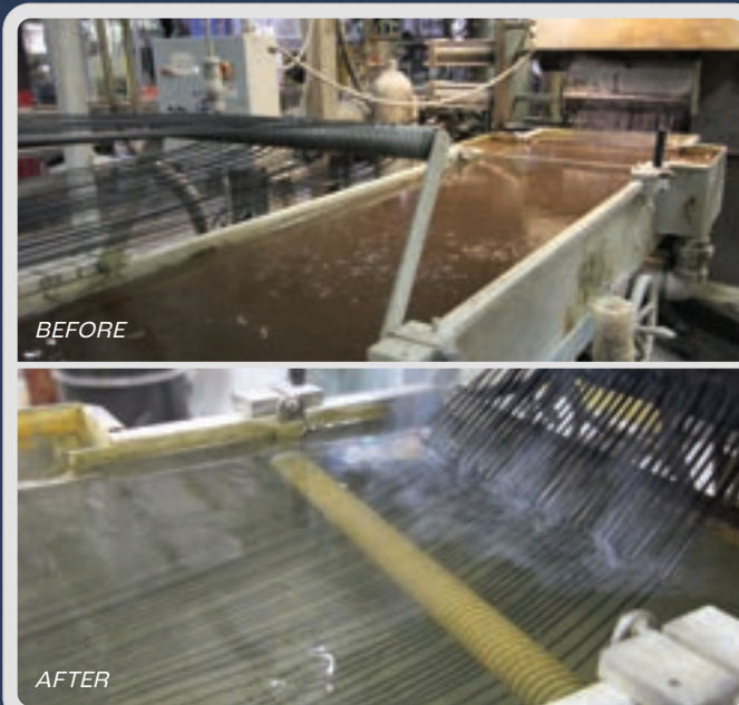
Extrusion baths before and after installation of Armstrong Nanobubble Generator (3/4"x1.5").
